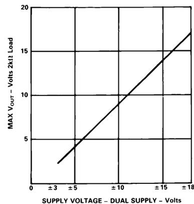
Figure 3. AD637 max  $V_{OUT}$  vs. Supply Voltage
