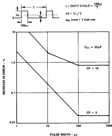
Figure 11. AD637 Error vs. Pulse Width Rectangular Pulse
