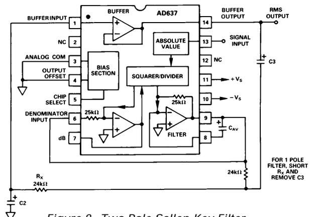
Figure 8. Two Pole Sallen-Key Filter
