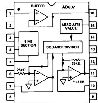
The AD637 is available in two accuracy grades (J, K) for commercial (0°C to +70°C) temperature range applications; two accuracy grades (A, B) for industrial (-40°C to +85°C) applications; and one (S) rated over the -55°C to +125°C temperature range. All versions are available in hermetically-sealed, 14-pin side-brazed ceramic DIPs as well as low cost cerdip packages. A 16-pin SOIC package is also available.
