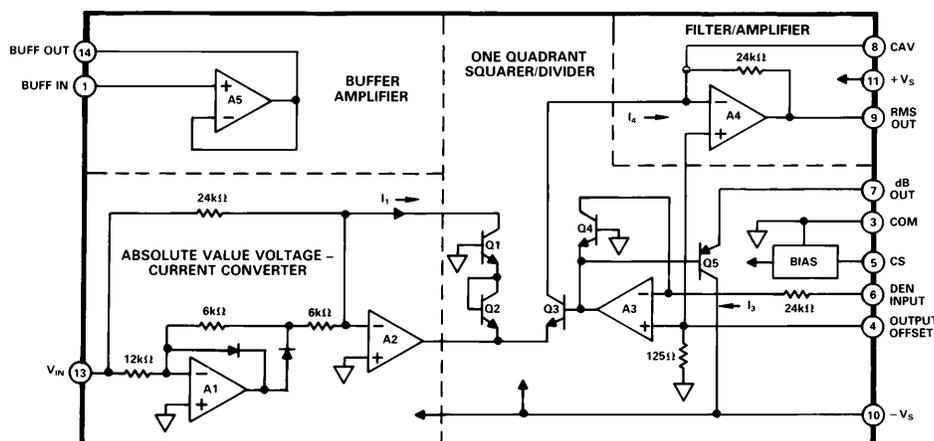
Figure 1. Simplified Schematic
