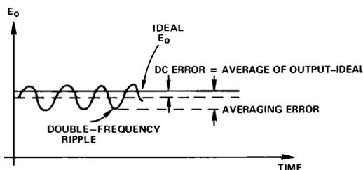
Figure 6. Typical Output Waveform for a Sinusoidal Input
