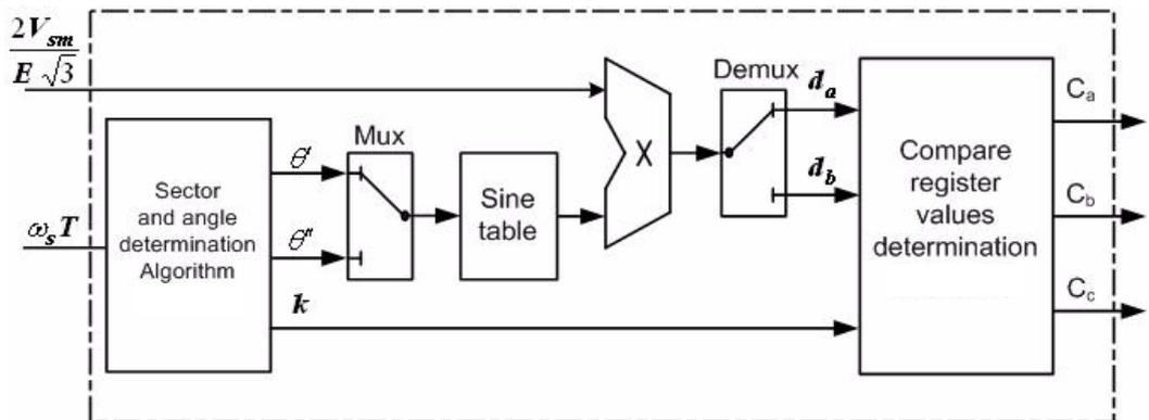
**Figure 4-8.** Block diagram of the complete control system.
